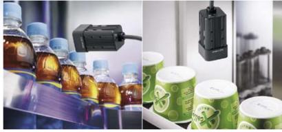
The ZFV verifies the correct position of the cap to secure proper closure of the bottle.
