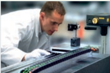
Precision measurement with laser interferometer for quality assurance to create the data for stage mapping.
