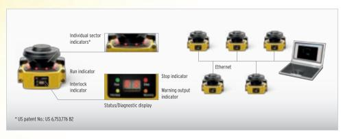
Simple monitoring of several OS32C units is achieved by integrated Ethernet communication for programming and maintenance. Clear maintenance information is given by sector indicators for easy recognition of which sector is blocked and the OS32C's status is given by a 7-segment display.
