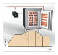
In time-based process applications, banks are used to hold PID and alarm values. They can also hold soak times as another way of creating an SV program.
