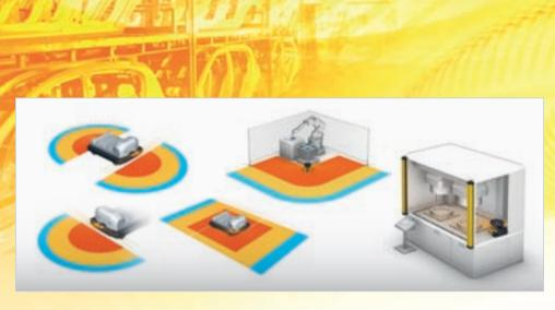
Flexibility of installation is ensured by 70 field sets of safety zone and warning zone combinations covering complex layouts of AGV routes in mobile applications.
