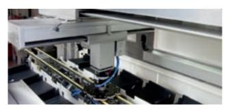
Omron's high speed linear motor slider system for precise sorting and handling of wafers
