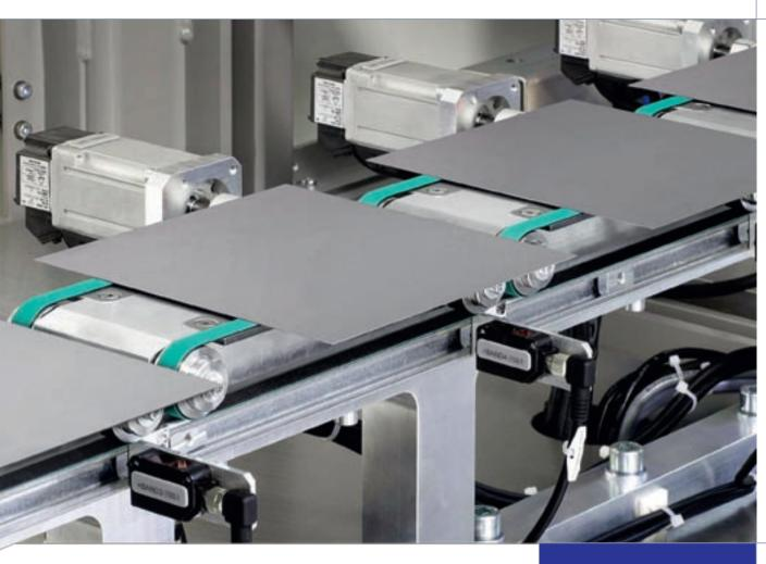
Wafer conveyor controlled by G5 servo motors with EtherCAT motion bus and optical E3Z family sensor
