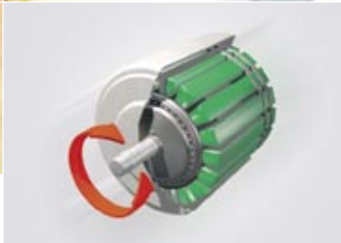
The principle of the AC servomotor: the stator and the rotor rotate in the same plane.
