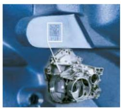
Data Matrix code directly applied to a gearbox
