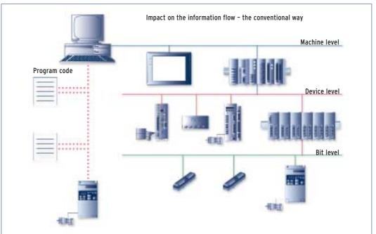
Figure 2: Impact of the information flow - the conventional way: Interfacing from one communication layer to another is done by manualy defined routing tables.
