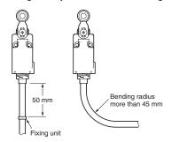
When wiring, be sure to prevent penetration of a liquid such as water or oil through the cable end.
