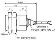
Note 1. 4-dia. vinyl-insulated round cable with 3 conductors (Conductor cross section: 0.3 mm²; Insulator diameter: 1.3 mm), Standard length: 2 m
