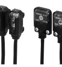
The side-view type has realized long, 1 m distance detection. Furthermore, it can detect a small, 0.5 mm or less dia. work with a pin-point beam (when slit is fitted). The visible light spot and narrow-visibility beam ensure a stable detection of lead frames and chip parts.
