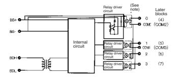
Note: The G3DZ-2R6PL Power MOS FET Relay is inserted into this portion of the SRT2-ROF08 and SRT2-ROF16.
