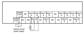
Note: The inputs of the DRT1-TS04 are insulated from one another and so consideration of input circuits is not required.
