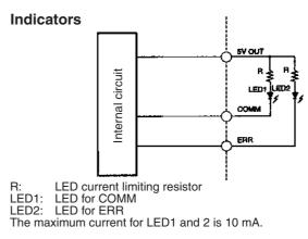
The 5-V Output Terminals have positive power supplies (maximum output current of 20 mA) for the ERR and COMM LEDs. Recommended LED colors are red for ERR and yellow for COMM.
