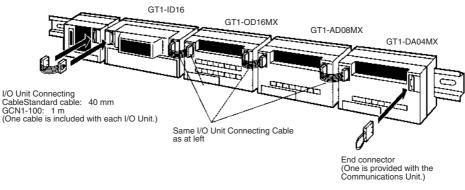
To connect the units to each other, use the with the I/O unit supplied connecting cable. Insert the end connector, which is delivered with the communication unit in the second communications connector of the last I/O unit as bus terminator.
