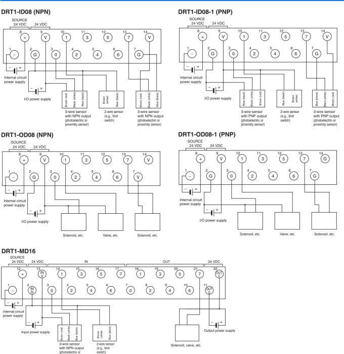
Note: Wire colors have been changed in accordance with revisions to JIS standards for photoelectric and proximity sensors. The previous colors are given in parentheses.
