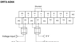
Note: With using a current input, always short the V+ and I+ terminals. (Use the shorting bar provided with the Unit.)
