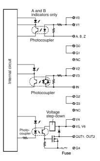
Be sure to connect Molex connectors for analog output wires and connect the wires as shown below.
