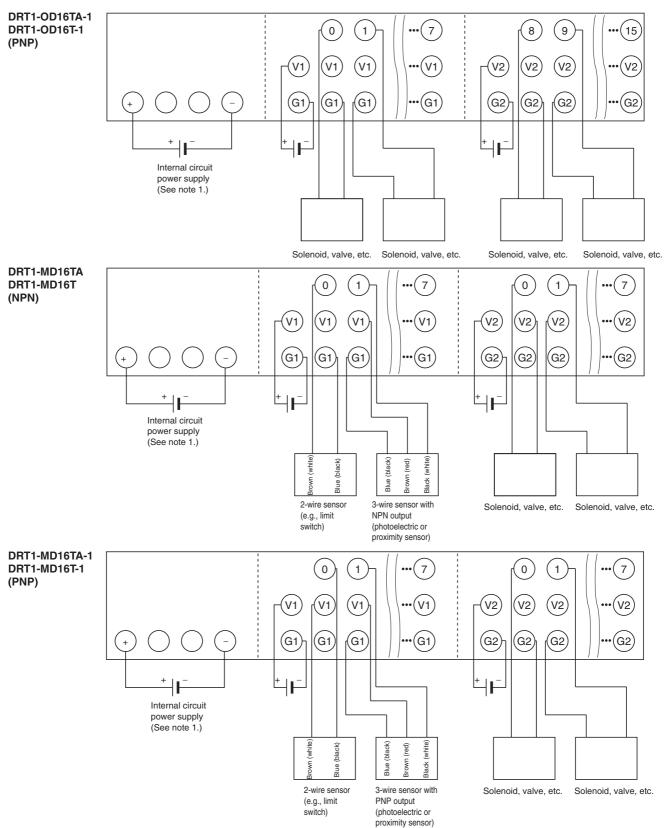
Note: 1. Internal circuit power supply wiring is not required for DRT1-D16TA(-1) models.
