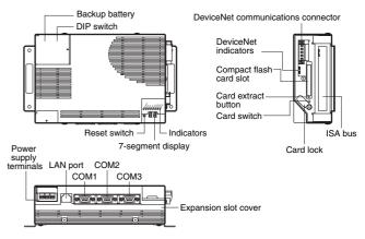
• Expandable Controller with DeviceNet support
