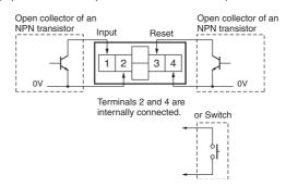
Note: 1. Residual voltage in the output section of Proximity Sensors or Photoelectric Sensors becomes less than 0.5 V because the current flowing from terminals 1 or 3 is small thus allowing easy connection.
