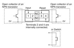
Note: 1. Residual voltage in the output section of Proximity Sensors or Photoelectric Sensors becomes less than 0.5 V because the current flowing from terminals 1 or 3 is as small as approx. 10  $\mu A$ , thus allowing easy connection.
