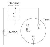
Operates with PNP transistor ON
