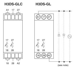
Note: DC supply voltage does not require the designation of polarity.
