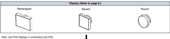
Note: Use IP40 Displays in combination with IP40 Cases and use IP66 oil-resistant Displays in combination with IP66 oil-resistant Cases. The Display has a legend plate built in.
