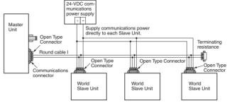
Before connecting the power supply, first connect a DCN4-TB4 Open Type Connector to the communications connector to convert it to a screw terminal block.
