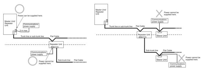
• Use separate power supplies for the Master Unit trunk line and for each sub-trunk line (i.e., for the trunk line on the Master side of the Repeater Unit and the sub-trunk line on the Slave side).
