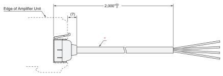
\*4-dia. cable with 4 conductors, Standard cable length: 2 m (Conductor cross-section: 0.2 mm² (AWG24), Insulation diameter: 1.1 mm)
