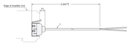
\*4-dia. cable with 2 conductors, Standard cable length: 2 m (Conductor cross-section: 0.2 mm² (AWG24), Insulation diameter: 1.1 mm)
