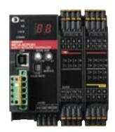
The just 90mm wide housing of the controller offers 16 (8 redundant) safety inputs and 8 solid state outputs with 500mA rating and self test. Four additional test pulse outputs ensure crosstalk and short circuit detection for the input channels. All in- and outputs comply with IEC 61131-2 (type 2).
