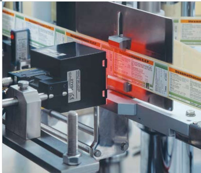
▶ A thermal printer prints variable durability dates and batch numbers onto the labels of a pharmaceutical product. The F250 intelligent sensor then examines these dates. The test station can be speedily and easily set up for other label formats.
