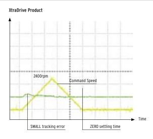
Small tracking error, zero settling time.
