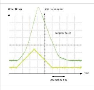
▲ Large tracking error, long settling time.
