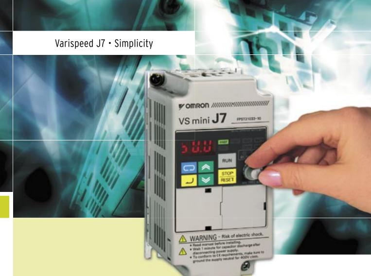
Simplicity and cost effectiveness are the key design features for the J7. Using Volts/Frequency control with on-line torque compensation the drive provides 100% torque down to 1.5Hz. The J7 has a built-in speed setting potentiometer, 4 configurable inputs, one configurable relay output as well as a multi-function analogue output.
