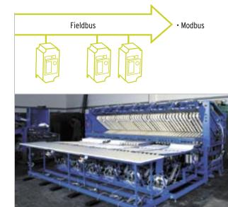
6-track folding machine for large laundry facilities: frequency inverter J7 allows variable speeds on the different track.
