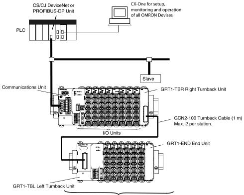
Up to 64 I/O Units can be connected to a Communications Unit.
