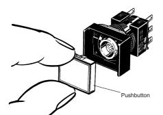
2. To attach the Pushbutton, push until it clicks into place.
