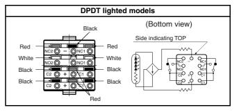
· Voltage-reduction lighting models with Screw-Less Clamps (A16L-T1-2S, A16L-T2-2S) incorporate voltage-reduction circuits.
