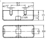
**Note: 1.** The Cover has five holes for easy lead wire connections.
