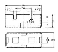
**Note: 1.** The Cover has six holes for easy lead wire connections.
