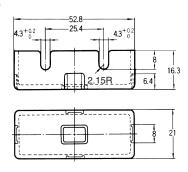
Note: The Cover has five thin, easy-to-separate portions for easy lead wire connections.
