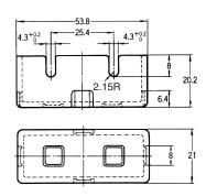
**Note:** The Cover has six thin, easy-to-separate portions for easy lead wire connections.
