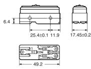
Appropriate terminal screw tightening torque: 0.78 to 1.18 N·m {8 to 12 kgf·cm}.
