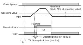
Note: The power ON lock prevents unnecessary alarms from being generated during the instable period when the power is first turned on. There is no relay output during timer operation.
