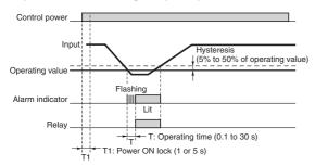
**Note:** The power ON lock prevents unnecessary alarms from being generated during the instable period when the power is first turned on. There is no relay output during timer operation.
