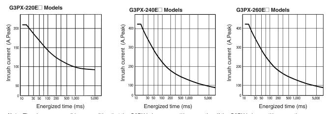
**Note:** The above are possible on condition that the G3PX is in non-repetitive operation. If the G3PX is in repetitive operation, reduce the applied current to half.
