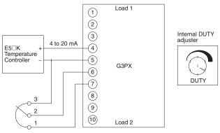
G32X-V3K External Variable Resistor (3  $k\Omega$ ) for duty setting
