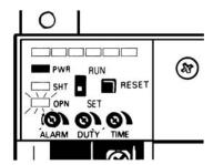
4. Set the RUN/SET switch to RUN. When all settings have been finished, the OPEN indicator is OFF.
