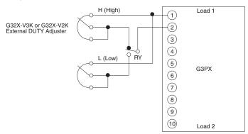
**Note:** 1. A temperature controller with relay output or a single relay can be used with the G3PX in two-position (high-and low-position) control, in which case the relay contact current is 30 mA at 12 VDC with the External DUTY Adjuster set to 0  $\Omega$ .
