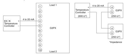
Note: Two G3PX models can be connected in series to OMRON's single Temperature Controller (with an internal impedance of 600  $\Omega$ ) with a current output.
