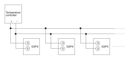
3. A Temperature Controller (with a relay output) is used to vary the duty of G3PX.
