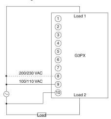
Note: Use a single power supply for the G3PX and the load.
