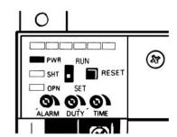
Adjust the sensitivity. Turn the ALARM adjuster and set to the position where the OPEN indicator is lit. Stop turning the ALARM adjuster as soon as the indicator is lit to complete the setting.
