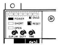
Note: When resetting, leave power supply terminals 10 to 9 or 8 ON.
