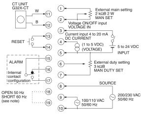
Note: Open the terminals for 50 Hz or short-circuit the terminals for 60 Hz. When the product is shipped, the terminals are short-circuited using a short-circuiting bar to set to 60 Hz. When using at 50 Hz, remove the short-circuiting bar.
