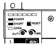
Note: When the G3PX detects a short-mode failure, all LEDs of the Level indicator and red SHORT indicator are lit. When you use a breaker to disconnect the load with the relay output, all LEDs of the Level indicator will be OFF regardless of the input to the G3PX.
