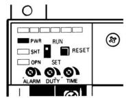
Note: 1. The G3PX can control any part of the phase as long as the controlled phase is approximately  $1/6\pi$  or more in width.
