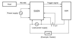
**Note:** Connect a power supply with the same phase as the SSRs to the load power supply terminals on the G3ZA.
