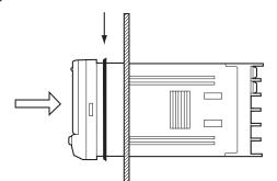
**3.** Fit the adaptor into the grooves on the left and right sides of the rear case, then push it until it contacts the panel to secure the K3MA-F.
