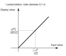
When displaying a flowrate (e.g., in l/min or l/h), make the scaling settings after confirming the I/O characteristics of the flowrate sensor. There are flowrate sensors that output analog signals. If this kind of flowrate sensor is used, consider using the K3MA-J.
