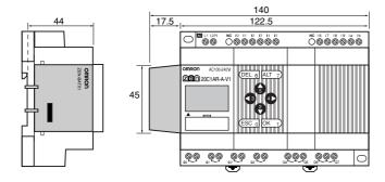
Expansion I/O Units (4 inputs, 4 outputs, 8 I/O)
