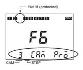
Set the cam number to be protected (and not displayed) to 3 with the CAM Keys  $\pm$  and then press the <u>WRITE</u> Key. The output display will go out.
