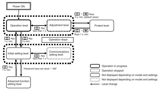
Note: Of these levels, the initial setting level, communications setting level, and advanced function setting level can be used only when operation has stopped. Control output is stopped when these three levels are selected. When switched back to the operation level from one of these levels, operation will start.
