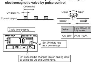
Refer to Input/Output Mode Settings on page D-50 for information on ON/OFF-duty adjustable flicker mode operation.
