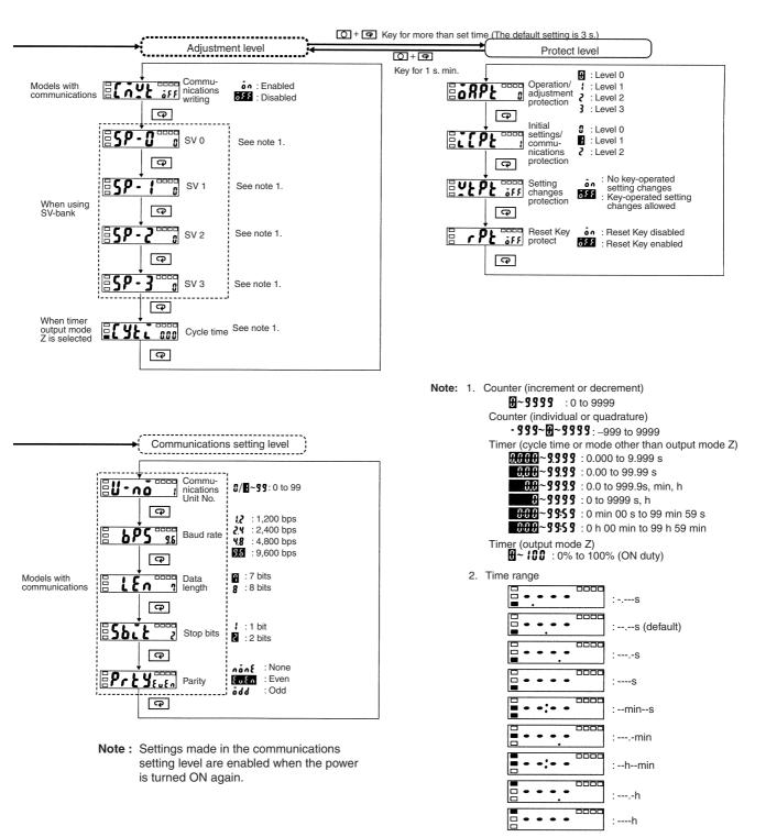
3. Displayed when level 0 is selected for initial setting/ communications protection in the protect level.
