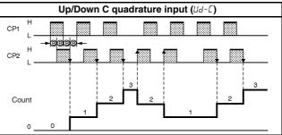
Note: 1. (A) indicates the minimum signal width and (B) requires at least 1/2 the minimum signal width. If these conditions are not met, a counting error (+1 or -1) may occur.
