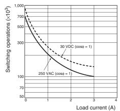
Reference: A maximum current of 0.15 A can be switched at  $125 \text{ VDC} (\cos \phi = 1)$  and a maximum current of 0.1 A can be switched if L/R is 7 ms. In both cases, <u>a life of 100,000 operations can be expected</u>. The minimum applicable load is 10 mA at 5 VDC (failure level: P).
