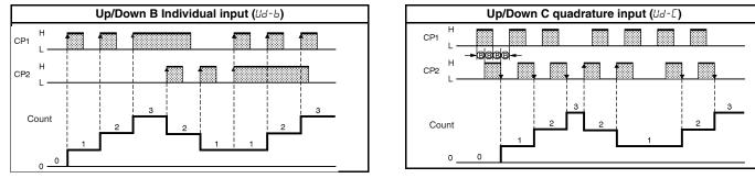
Note: 1. (A) indicates the minimum signal width and (B) requires at least 1/2 the minimum signal width. If these conditions are not met, a counting error (+1 or -1) may occur.
