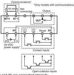
Note: (2) and (6) are connected internally. Do not use unused terminals as relay terminals.
