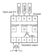
The power supply and input circuit are not insulated. Terminals 1 and 6 of the H5CX-ASD are connected internally.
