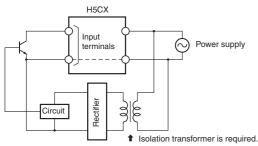
Make sure that the voltage is applied within the specified range, otherwise the internal elements of the Timer may be damaged.
