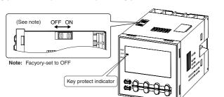
When the key-protect switch is set to ON, it is possible to prevent setting errors by prohibiting the use of certain operation keys by specifying the key protect level (KP-1 to KP-5). The key protect indicator is lit while the key-protect switch is set to ON.
