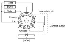
The power supply and input circuit of the H5CX-A11 have basic insulation. The power supply and input circuit of the H5CX-A11D are not insulated. Terminals 2 and 3 of the H5CX-A11D are connected internally.
