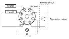
The power supply and input circuit are not insulated. Terminals 1 and 2 of the H5CX-L8SD are connected internally.
