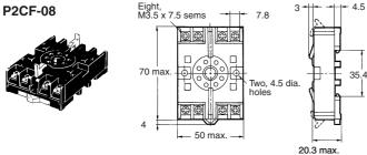
P2CF-08-E (Finger Safe Terminal Type) Conforming to VDE0106/P100
