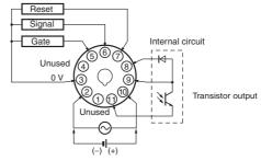
The power supply and input circuit of the H5CX-A11S have basic insulation. The power supply and input circuit of the H5CX-A11SD are not insulated. Terminals 2 and 3 of the H5CX-A11SD are connected internally.
