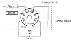
The power supply and input circuit are not insulated. Terminals 1 and 2 of the H5CX-L8D are connected internally.
