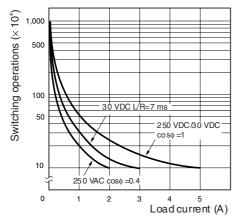
Reference: <u>A maximum current of 0.15 A can be switched at 125 VDC (cosφ=1)</u> and a maximum current of 0.1 A can be switched if L/R is 7 ms. In both cases, <u>a life of 100.000 operations can be expected</u>. The minimum applicable load is 10 mA at 5 VDC (failure level: P).
