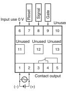
The power supply and input circuit are not insulated. Terminals 1 and 6 of the H5CX-AD are connected internally.
