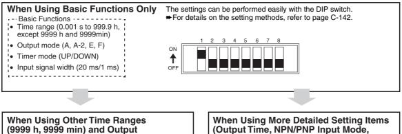
Modes (A-1, A-3, b, b-1, d, and Z) All the functions can be set with the operation keys. ➡For details on the setting methods, refer to page C-143.
