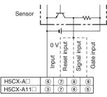
Operate with transistor OFF
