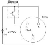
Operates with PNP transistor ON
