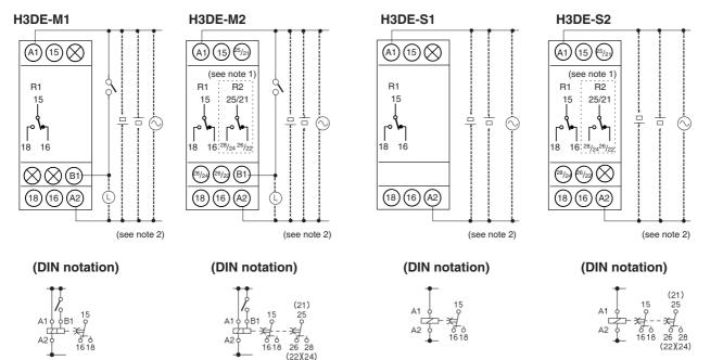
Note: 1. The relay R2 can be set to either instantaneous or time-limit contact using the switch located on the bottom of the Timer.
