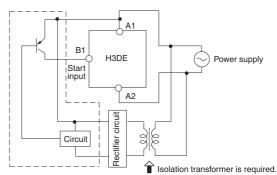
The H3DE-H has a large inrush current; provide sufficient power supply capacity. If the power supply capacity is too small, there may be delays in turning ON the output.
