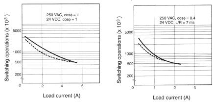
Reference: A maximum current of 0.6 A can be switched at 125 VDC ( $\cos\phi = 1$ ). Maximum current of 0.2 A can be switched if L/R is 7 ms. In both cases, a life of 100,000 operations can be expected. The minimum applicable load is 1 mA at 5 VDC (P reference value).
