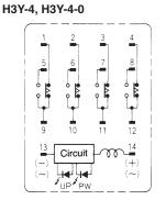
Connect the DC power supply to terminals 13 and 14 according to the polarity marks.
