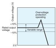
Note: Do not turn ON the power again until the cause of the overvoltage has been removed.
