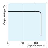
Note: Do not allow the short-circuited or overcurrent state to continue for more than 20 s, otherwise it may damage the element.
