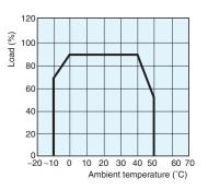
Note: If there is a derating problem, use forced air-cooling. The ambient temperature is specified for a point 50 mm below the power supply.
