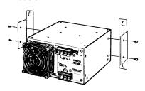
Note: Mount the Unit 28 mm away from the mounting surface in order to provide air ventilation on the rear side.
