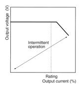
Note: Do not continue using the S8PS under short-circuited or overcurrent conditions for longer than 20 seconds, otherwise the internal elements of the S8PS may be damaged or broken.
