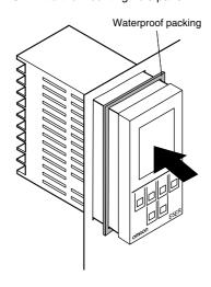
3. Insert the mounting brackets into the grooves on the top and bottom of the rear case.
