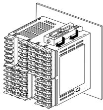
4. Tighten the screws on the mounting brackets alternately, keeping an even balance, until the ratchet stops tightening.
