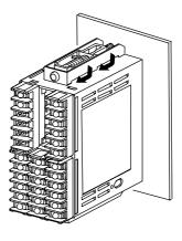
**4.** Tighten the screws on the mounting brackets alternately, keeping an even balance, until the ratchet stops tightening.
