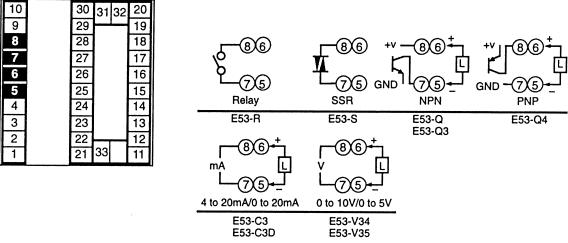
With E53-V Output Units, approx. 2 V is output for one second after the power is interrupted.
