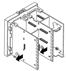
2. Insert the Option Units into the sockets for options 1 to 3. The following diagram shows the relationship between the Option Units and mounting positions.
