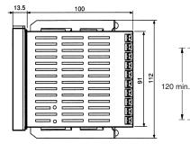
Note: 1. Recommended panel thickness is 1 to 8 mm. 2. Maintain the specified vertical and horizontal mounting space between each Unit. Units must not be closely mounted vertically or horizontally.
