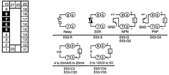
With E53-V $\square$  Output Units, approx. 2 V is output for one second after the power is interrupted.
