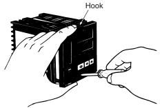
2. Draw out the internal mechanism while holding the left and right sides of the front panel.
