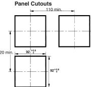
Note: 1. Recommended panel thickness is 1 to 8 mm. 2. Maintain the specified vertical and horizontal mounting space between each Unit. Units must not be closely mounted vertically or horizontally.
