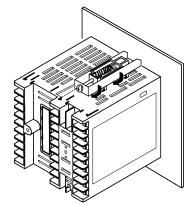
**3.** Tighten the mounting bracket screws on the upper and lower parts of the E5AK in small increments alternately and equally until the ratchet start to slide.
