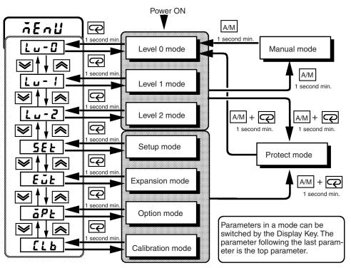
Note: The control of the Digital Controller is reset when the Digital Controller is in setup, expansion, option, or calibration mode, in which case the control and auxiliary outputs are OFF. The reset condition will be canceled when the Digital Controller is in any mode other than the above.
