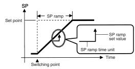
The change rate during the SP ramp is specified by the "SP ramp set value" and "SP ramp time unit" parameters. At the "SP ramp set value" default "0," the SP ramp function is disabled.
