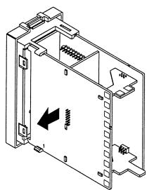
2. Insert the Option Unit into the socket for option 1. The following diagram shows the relationship between the Option Unit and mounting position.
