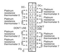
Make sure there in no difference in resistance among the three conductor of each platinum resistance thermometer used with the E5ZE.
