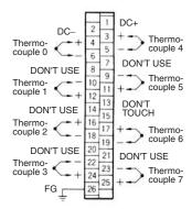
A thermocouple has polarity. Connect thermocouples to the terminal block correctly using compensating conductor that are suitable for the thermocouples.
