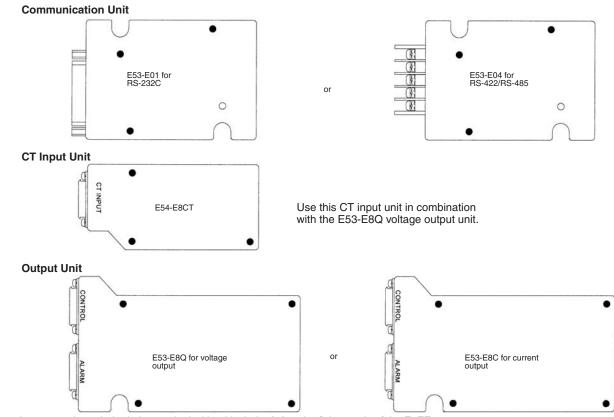
Tighten the screws through the holes marked with a black dot (●) to the fixing studs of the E5ZE.
