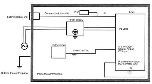
Note: 1. Place the power supply, filter, input sensor, I/O terminals, and communications cable inside the control panel when wiring them.
